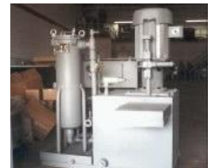
HIGH PRESSURE SKID- Deliver Clean High Pressure Coolant To Spindle
