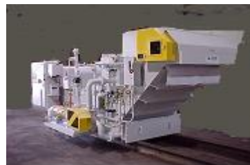
PUMPBACK TANK- Pump Chips and Coolant From Multiple Machines To a Single Central Filtration System
