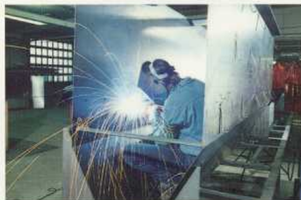
Flume & tank fabrication
